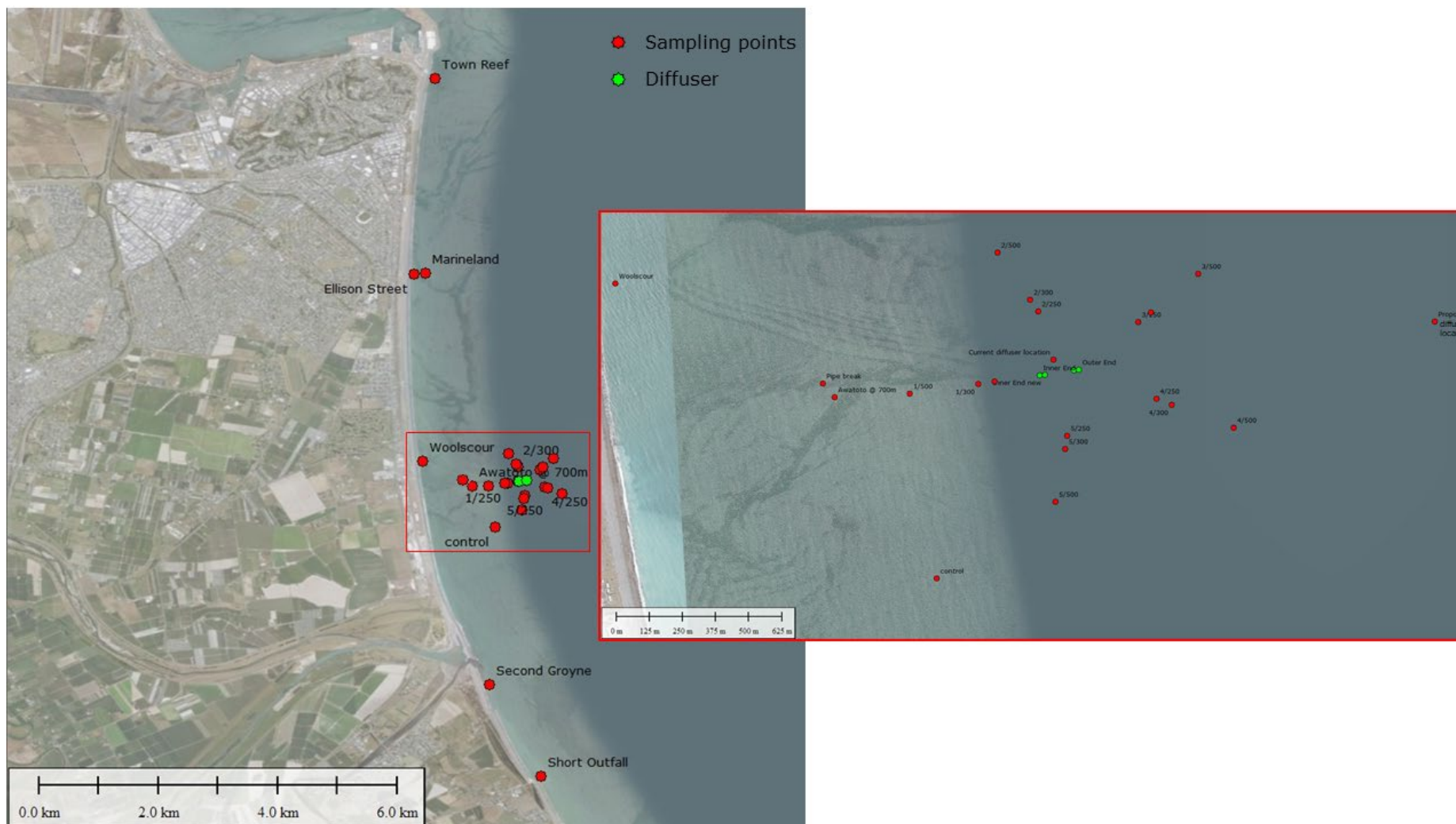
Figure 1.1 Location of the Napier City Wastewater Ocean Outfall. Green points indicate the current diffuser locations. The red circles show the locations where time series were extracted and give the locations of the scenarios modelled, given in Table 1.1.
